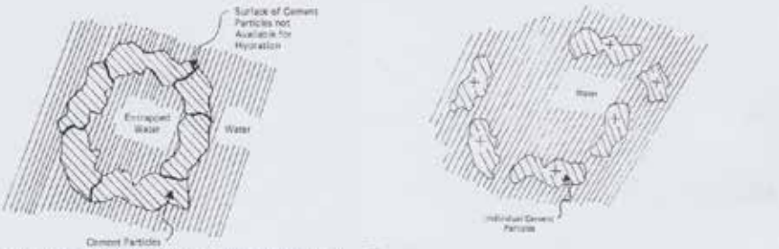
Figure 3-1: Cement particles in the absence of a dispersing agent.
